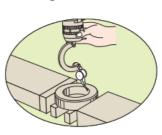
With Double Dial type, readings can be made easily even if gauge is turned 180 deg.
